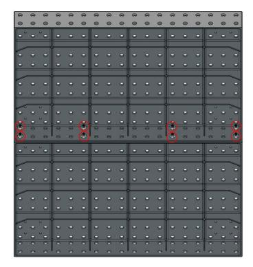
**STEP 3:** Install the legs (or other support system if the leg kit is not being used) and set the table onto the floor. Since the bolts were left slightly loose, the table surface should be concave.
