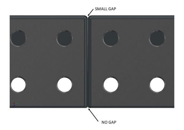
Before the blocks are bolted together, this gap must be filled to ensure that the top surface flatness is maintained. That is accomplished using the ArcFlat liquid shim bolt kit. These special bolts make it possible to inject liquid shim material (two part epoxy resin) into the joint immediately surrounding the bolt. Once the material is cured, the bolts can then be torque without the gap closing up.
